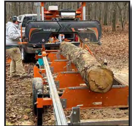
Photo 3: Salvaging green ash lumber.
