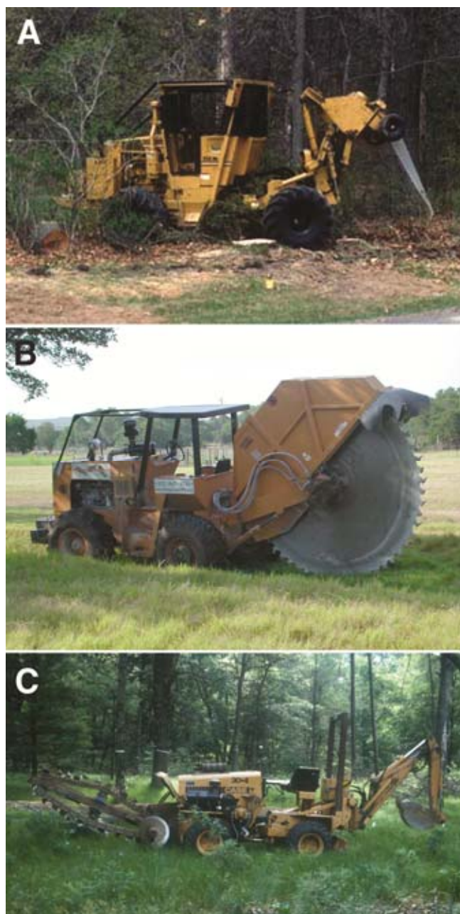
Fig. 9. Heavy equipment used to sever connected root systems around perimeter of oak wilt infection centers: A , vibratory plow commonly used in the Great Lakes States; B , rock-saw commonly used in Texas; and C , belt trencher machine occasionally used in northern states. Photo sources: A and C , J. Juzwicz; B , B. Moltzan.
