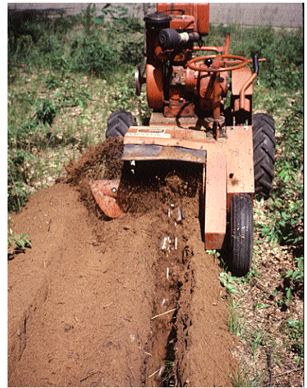
Example 3b. Oak wilt trenching.
