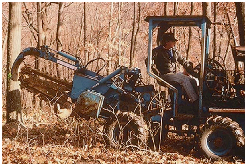
Example 3d. A trencher is a rubber-tired vehicle with a digging chain attached to the back. The chain moves along a boom, digging a trench and breaking root grafts as it is pulled through the soil.
